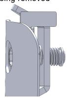
**CAUTION:** No treatment must be applied to the screw, no galvanizing, no painting, no baking.
