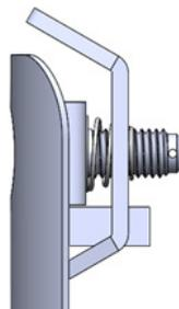
6. Insert the split pin and then bend both ends to prevent it from being removed
