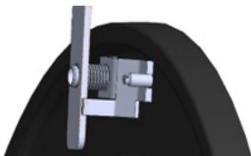
**5.** Tighten the M8 nuts and double-check the alignment when installing them.
