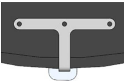
**2.** Drill the holes. The ones at the ends are to be drilled at Ø8mm and the central one at Ø14mm
